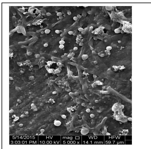
Fig 4:SEM confirming the formation of Biofilm on chitin flakes at 500 X
